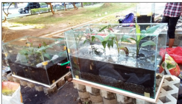
Figure 3. The model hybrid constructed wetlands system
